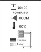
c. Move the cassette forward or backward from the paint surface to adjust to the best distance for curing. The distance data will be detected and shown on the display screen automatically. The measuring range is 20-120cm and beyond it is blind zone. The curing distance between the cassette and paint surface should be set according to the paint material and weather conditions (air humidity). Usually, keeping a distance of about 45cm from the paint surface is recommended.
