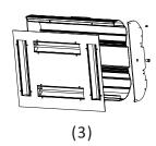
3. Remove the screws on the front panel to open it.
