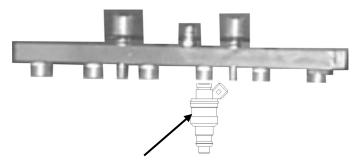
4.Please insert the pulse cable into the injector socket and mark the injectors in order.
