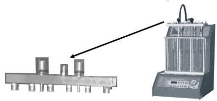
3. Fix the injectors that will be tested. First check the injector resistance value, this value can not exceed  $1\Omega$ , if the resistance value is above  $1\Omega$ , this injector must be replaced.
